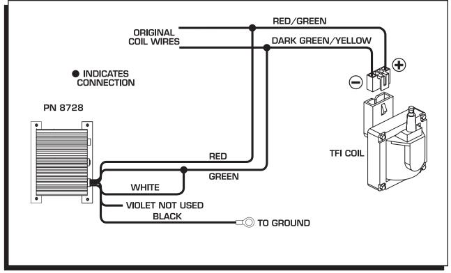
Figure 8 Wiring to a Ford TFI Ignition.
