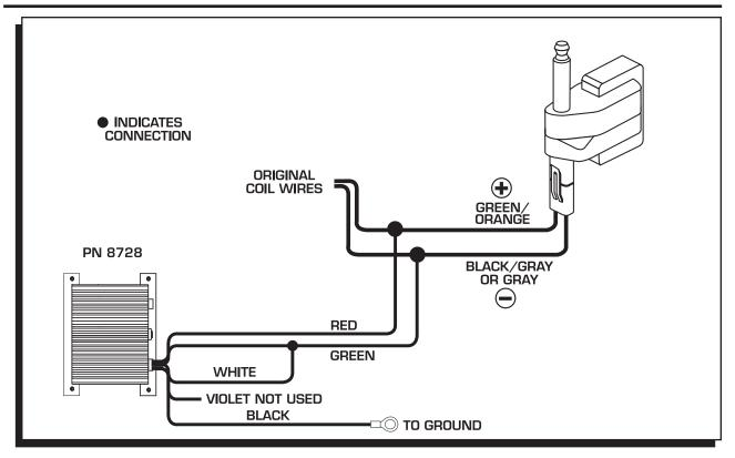
Figure 10 Wiring to a Late Model Dodge Ignition.
