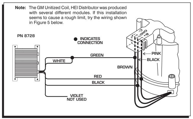
Figure 4 Wiring to a GM HEI Distributor, using the Module.
