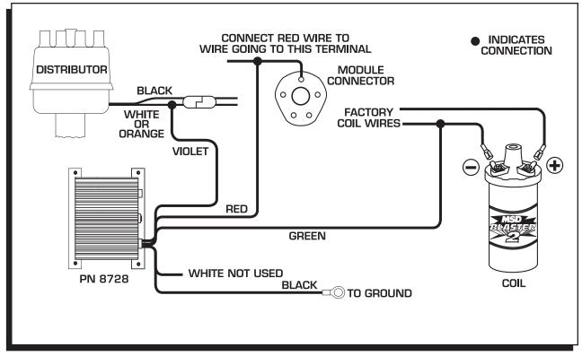
Figure 9 Wiring to a Chrysler Magnetic Pickup.
