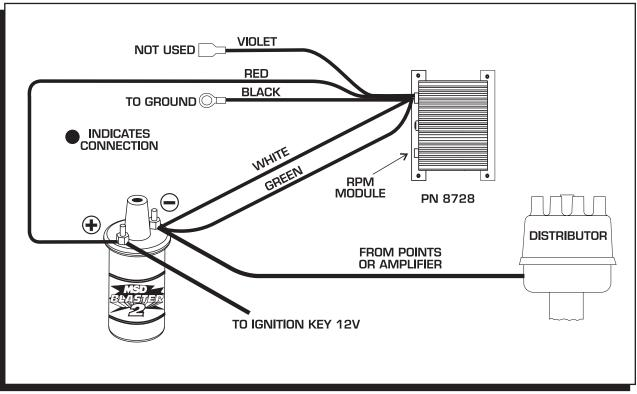
Figure 3 Wiring to a Points/Amplifier Ignition.
