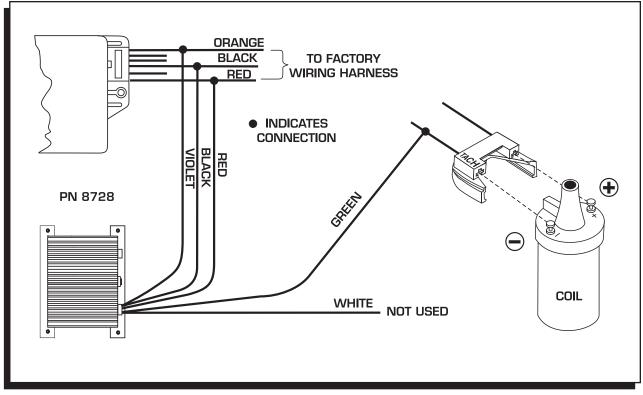
Figure 7 Wiring to a Ford Duraspark Ignition.
