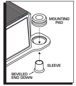
Figure 2 Installing the Vibration Mounts.
