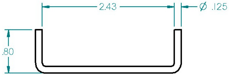
Figure 3. Clutch assembly wire dimensions. Not to scale.
