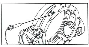
Illustration shows location of the breather assembly when installed.
